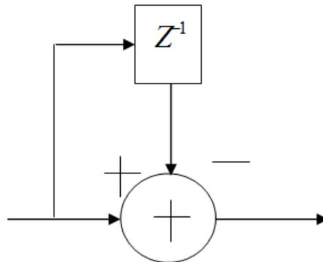
Figure 1.2:- Basic Comb Filter
