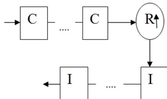
Figure 1.4:- CIC Interpolator Filter
