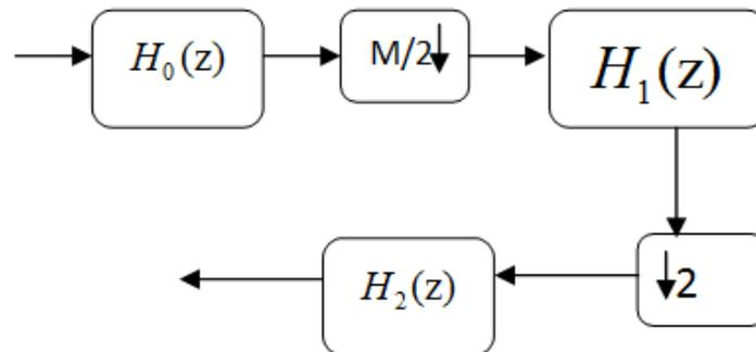
Figure 2.1:- Proposed Structure of CIC Filter
